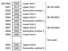
Note: An upper or lower limit can be set with integers in BCD mode and 5° increments in 360° mode. Subroutine numbers are set for interrupt processing.
