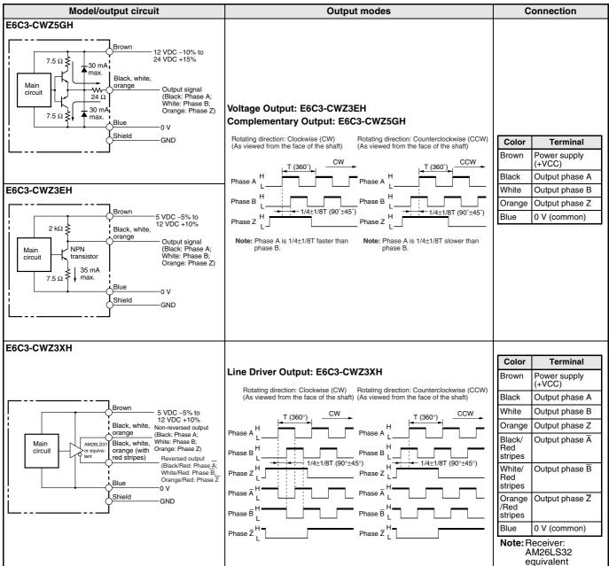
Note 1. The shield is not connected to the internal circuits or casing of the E6C3.
