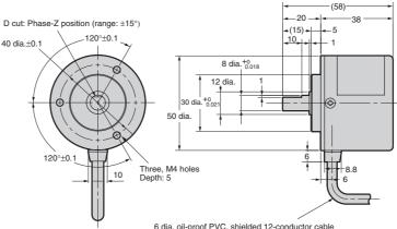
6 dia. oil-proof PVC, shielded 12-conductor cable (conductor cross-section: 0.2  $\rm mm^2;$  insulation diameter: 1.1 mm) Standard length: 1 m
